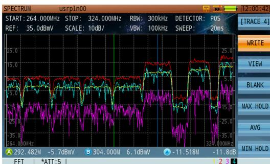
Four Traces Display Simultaneously
