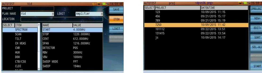
In the **Project** and **Location** fields, you can name the auto test project and the physical test address using the alphanumeric keypad. Highlight and click the **Plan Name** and **Limit** fields to select the desired channel plan and test point location for this project. (If you plan to import the output file into a pre-configured TWC Workbook, you may choose any arbitrary test point location.)
