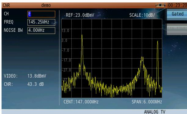
Typically, CCN measurements require that system engineers first measure the video carrier level (where the sync tip of the modulation is the absolute peak level); then remove the video modulation by shutting down the modulator - or simply remove the modulation from the carrier - to allow accurate noise measurement. Unfortunately, removing the modulation interrupts service.
