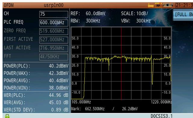
**Spectrum Measurement – Full-Band Spectrum**
