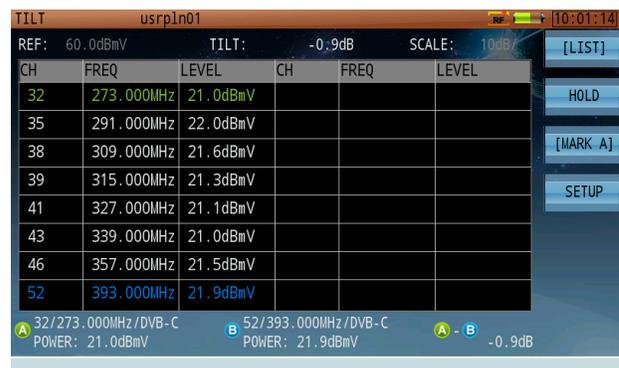
**Tilt Measurement – Channel Listing Display**
