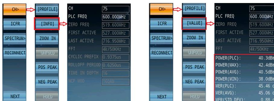
Press **CH>** (F1), **[INFO]** (F2) (above, left) to show the full channel info pane. Then press **[VALUE]** (F2 again) (above, right) to show power and MER statistics, which overlay part of the channel info pane. You can freely toggle between these view modes at any time.
