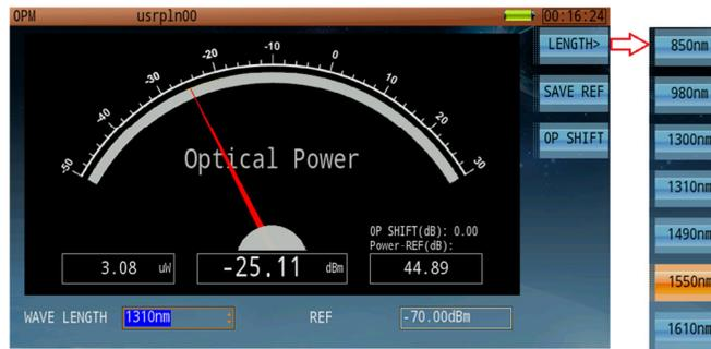
**Optical Power Meter Measurement Screen**
