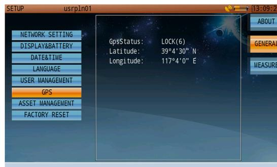
GPS coordinates are recorded at all times when a clear GPS positioning antenna has clear line of sight to the skies. The GPS coordinates are saved when a measurement is saved in "DATA" format, however, the GPS coordinates will not be displayed on a "Picture" file format.
